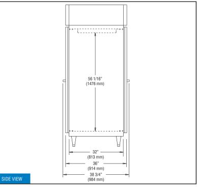
**IMPORTANT NOTE:** If the cabinet is located under a low ceiling, a <u>minimum</u> <u>clearance of 12" is required on</u> top and 3" on sides.
